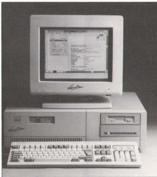
The Vanilla 386-20 is designed for file server and high-performance workstation applications.
